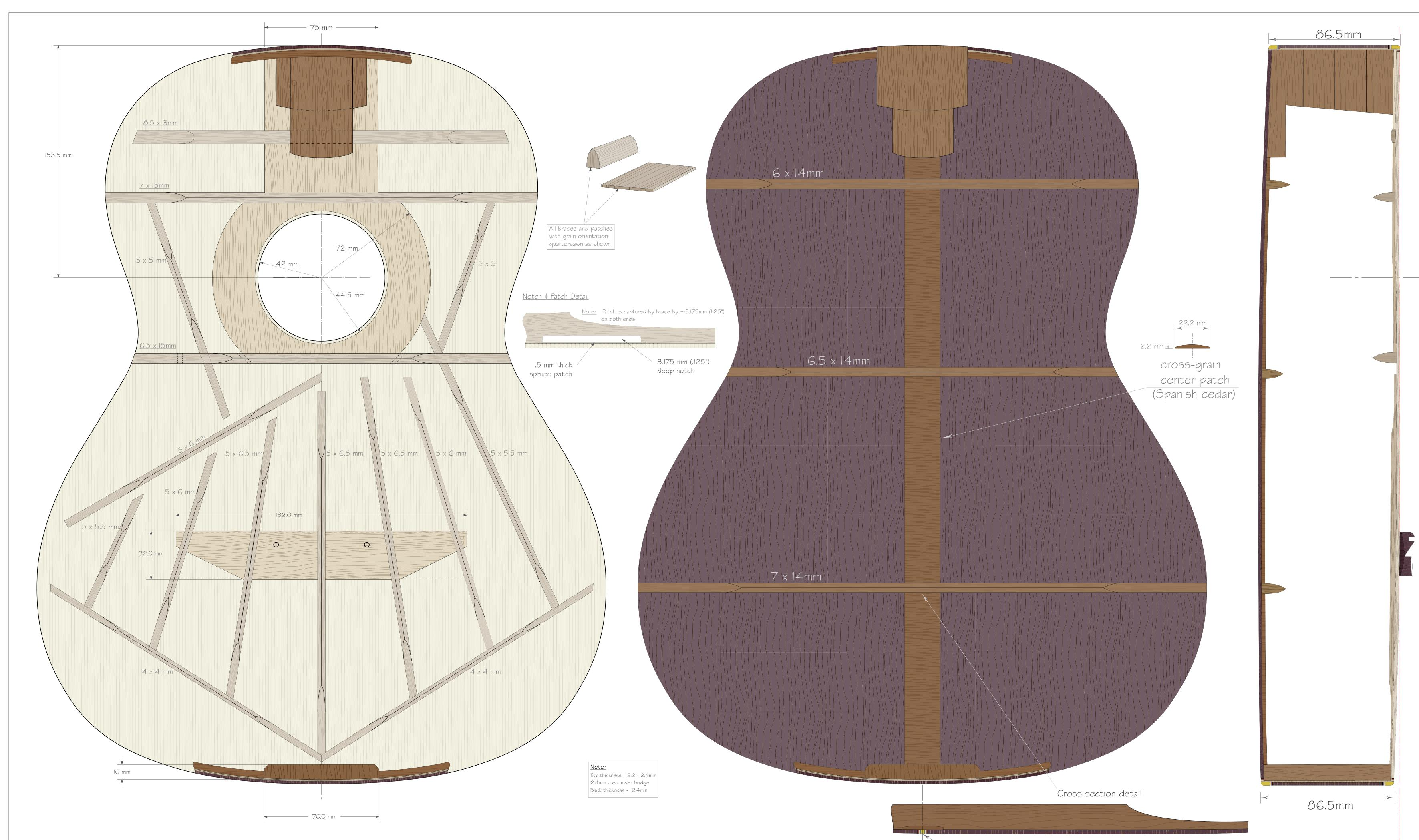
Back Strip sandwiched between the two halves
